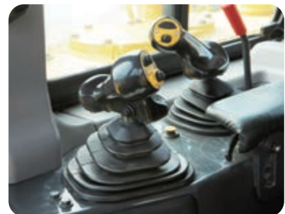
Blade control lever with auto-pitch and new ripper control lever with auto-return function
