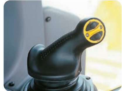
Commandes ergonomiques PCCS (Palm Command Control System)
