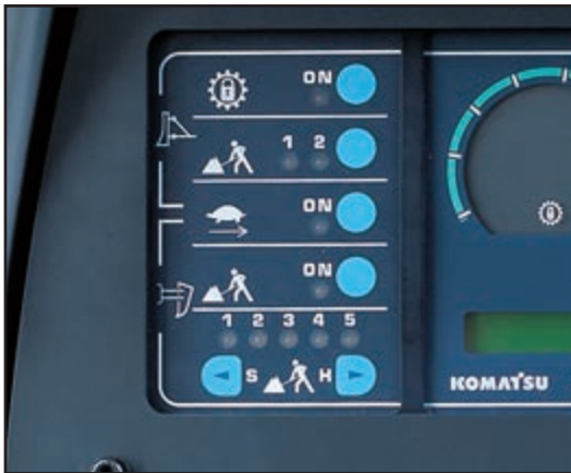
Track shoe slip control panel
