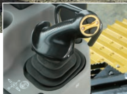
Commandes ergonomiques PCCS (Palm Command Control System)
