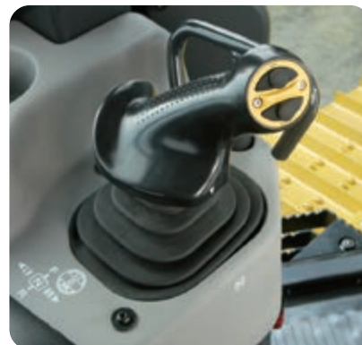
Commandes ergonomiques PCCS (Palm Command Control System)
