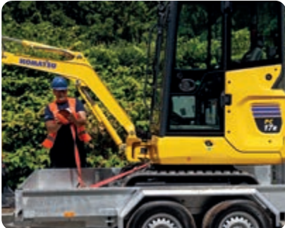
Tie down points on upper structure help to quickly secure the machine for transport
