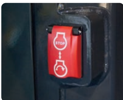
Secondary engine shutdown switch
