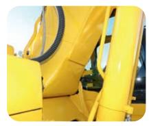
Cast boom foot and single piece boom plates
