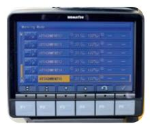
Komatsu Integrated Attachment Control (KIAC) for up to 15 tool presets for oil flow and pressure
