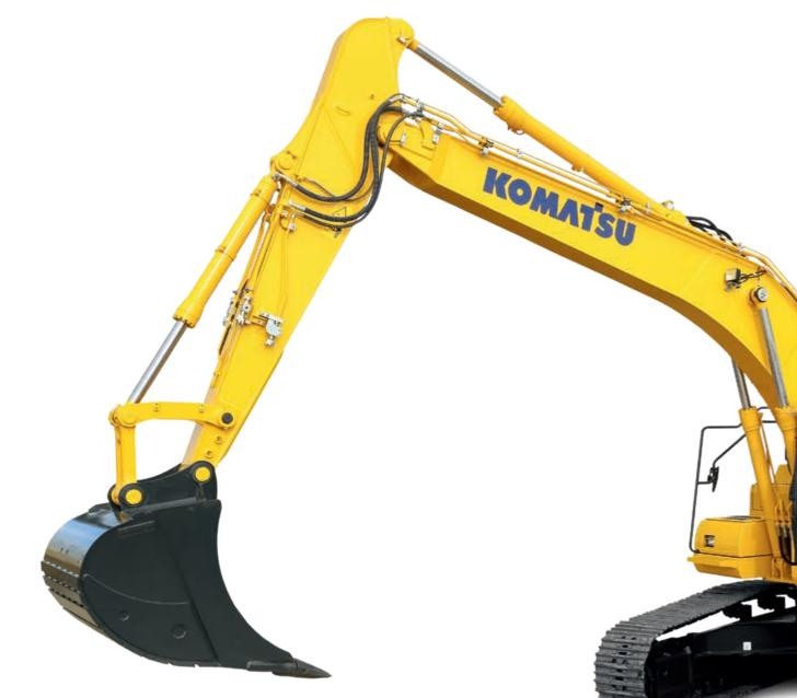
Engine power 159 kW / 213 HP @ 2050 rpm Operating weight PC290LC-11: 29950 - 32280 kg PC290NLC-11: 29850 - 32180 kg Bucket capacity max. 2.02 m<sup>3</sup>
