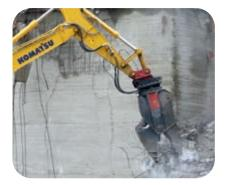
Two optional hydraulic lines to mount a variety of attachments
