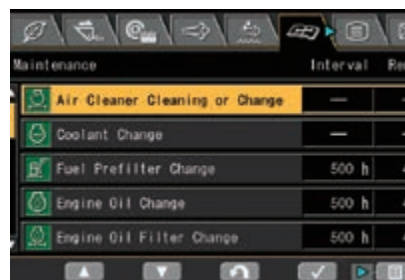
A multifunction monitor displays and controls a wealth of operational and maintenance information
