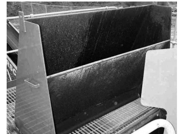
Roll in chute for transfer of material from screen to chutes, and ease of access for mesh
