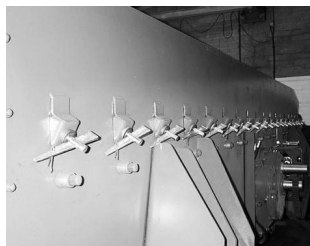
Side tensioned screenbox (Quick release wedges optional)
