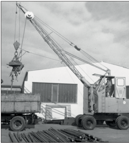
1962: Rope-driven S833 with elevated operator cab
