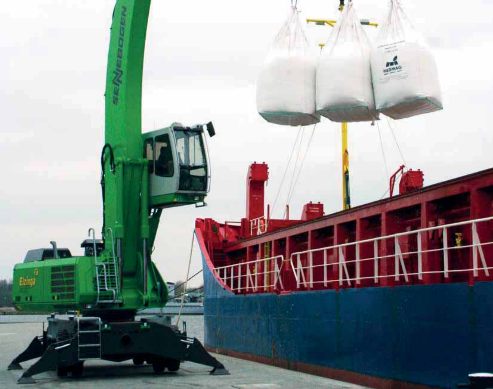
835 Mobile - B18 equipment, big bag handling; Netherlands 835 Mobil - Ausrüstung B18, Big Bag-Verladung; Niederlande
