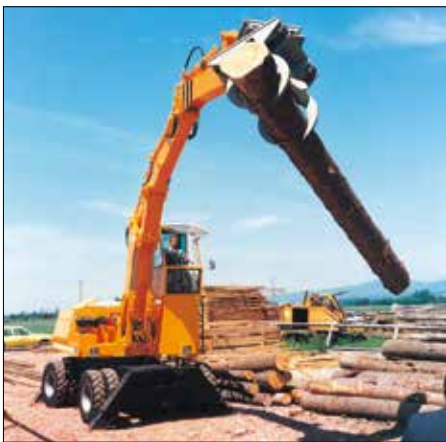
1974: Timber handling machine with elevated cab
