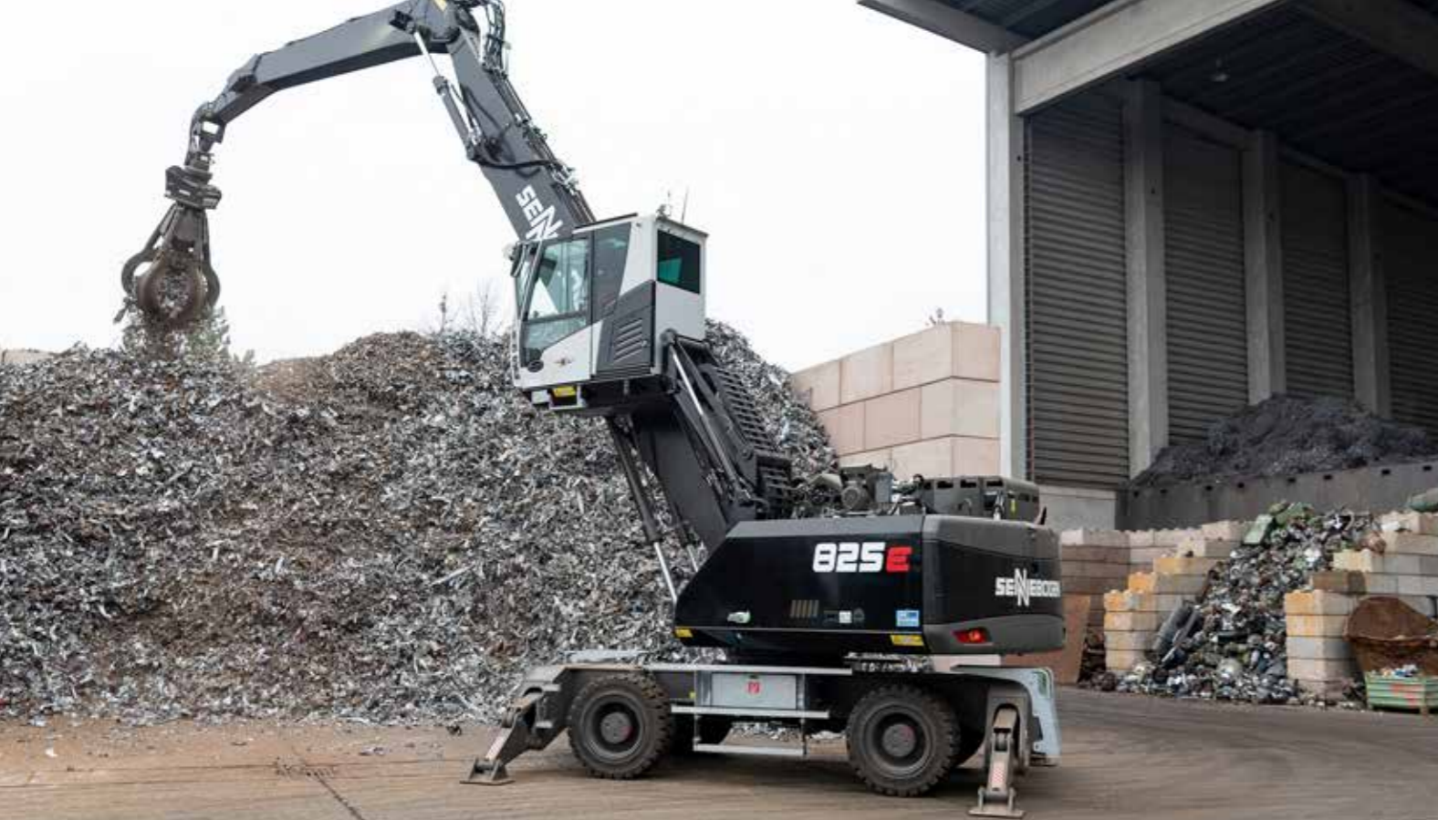
825 M - Scrap handling with orange peel grab; Germany
