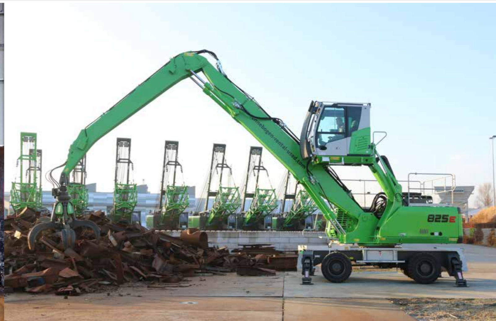
825 M - Mobile scrap handling with original SENNEBOGEN orange peel grab; Germany
