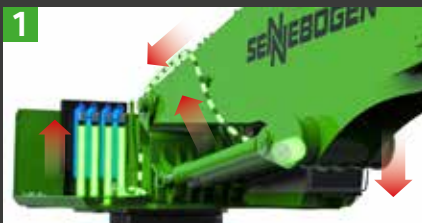
1 Boom lowers, gas compresses
